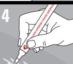
Very lightly dab the scratch. DO NOT DRAG TIP ACROSS THE SURFACE TO TOUCH-UP. Let dry for 20 to 30 minutes before applying a second coat if necessary. Replace cap after each use.
