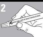
Apply **BASE COAT (A)** from touch-up pen first – two coats of **BASE COAT (A)** will be required.
