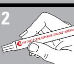
Apply **TOP COAT (B)** from touch-up pen – Only one coat should be required.
