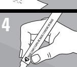
Very lightly dab a first coat in the scratch or chip. DO NOT DRAG TIP ACROSS THE SURFACE TO TOUCH-UP. You will notice that the paint has some transparency, the second coat will make it opaque. Replace cap after use.
